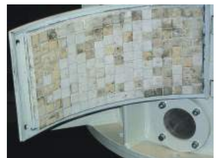
3. ALPHA with internal ceramic lining
