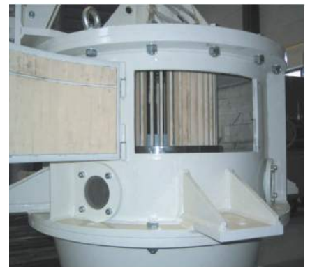
2. ALPHA 200CD for abrasive products with ceramic flaps
